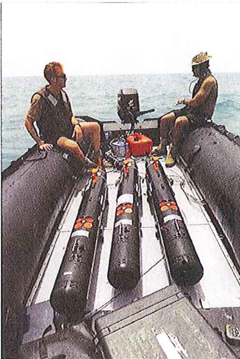
Divers from the USS Dextrous, a Navy MCM vessel, recover UUVs in the Persian Gulf.
