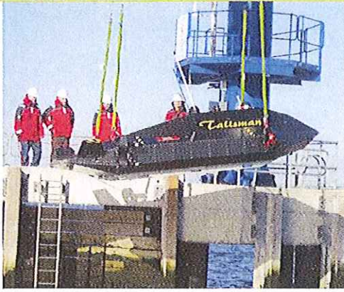
Talisman M from BAE can transport smaller UUVs for reconnaissance and minehunting missions.
