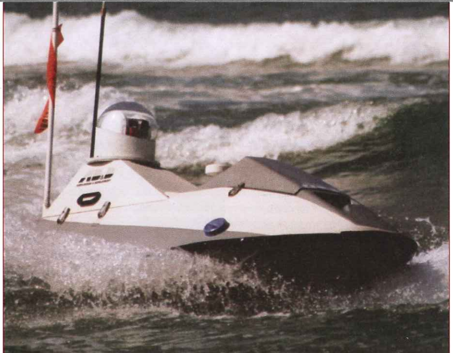
Elbit's Stingray is a high-speed USV, suitable for port and infrastructure security duties. (Photo: Elbit systems)
