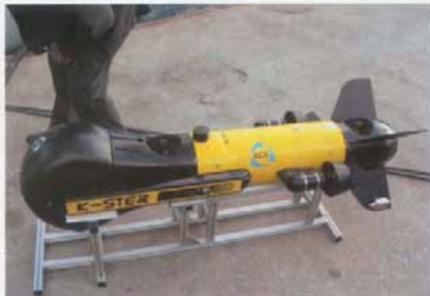
Fig. 5: It was a surprise to see how small ECA's K-ster mine destruction vehicle is, featuring the unique tilt-able head. K-ster was displayed as part of the TRIPARTITE Upgrade outside FS "Verseau".
