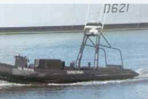
Fig. 10: One of many possible roles of SIREHNA's RODEUR unmanned surface vehicle (USV), seen here doing harbour surveillance alongside the "Chevalier Paul" (second-of-class HORIZON frigate) in Lorient. It benefits from the company's unique ship dynamic control features (motion and hull monitoring, motion stabilisation control and moving mass stabilisation system, wave control for dynamic positioning) which enable e.g. for the first time the stabilised lowering of the FLASH sonar from a USV.
