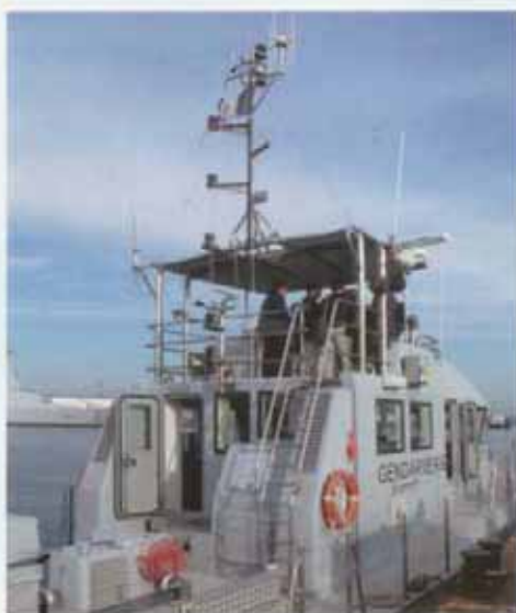
Fig. 9: The RPB 20 of Raidco Marine, seen here as a boat of the French Gendarmere, has been exported for use in many international markets. Its double-chine deep-V hull design provides excellent sea keeping with outstanding crew comfort.
